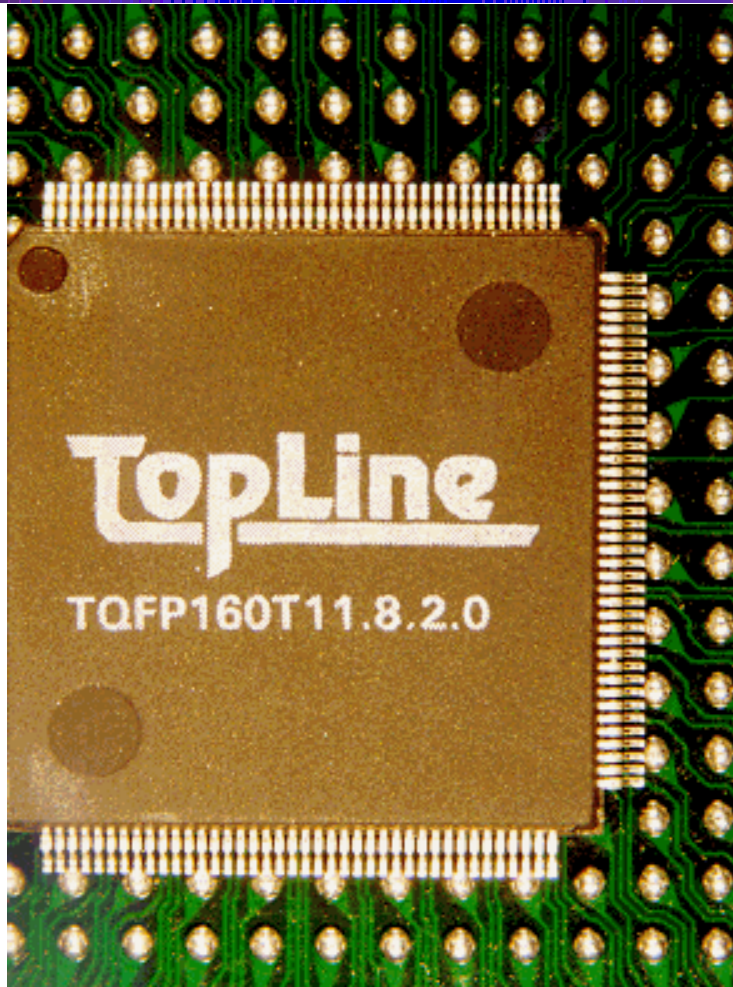
Figure 23.14 A 160-lead 0.3 mm pitch QFP placed on a grid of 1.5 mm pitch spheres (bottom side of a PBGA225)
